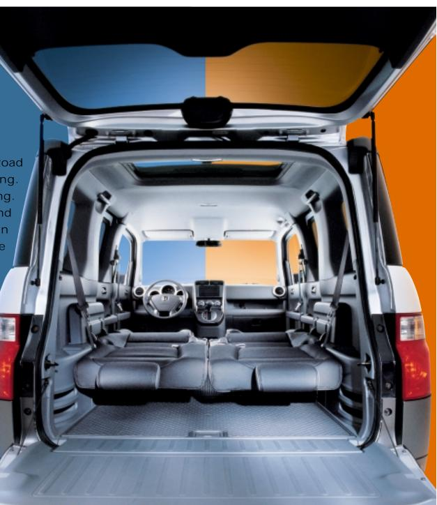
Throw in your muddy, snowy, sandy stuff. The waterproof and stain-resistant FXC<sup>™1</sup> (Fabric for Extreme Conditions) seating surfaces and a low, flat wipe-down urethane-coated utility floor can take the abuse. There are plenty of tie-down points to keep cargo secure, available seatback bungees for extra bits and a removable skylight (4WD) for even more breathing room.
