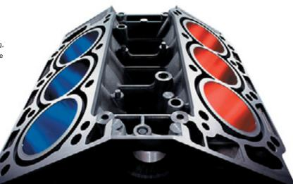
Cruise under light engine loads and VCM deactivates the three rear cylinders. The intake and exhaust valves remain closed, while fuel injection is paused. This can help deliver an EPA highway mileage rating of **28 mpg.**<sup>10,11</sup> Road trippers take note, that's a potential range of nearly **588 miles.**<sup>10†</sup>
