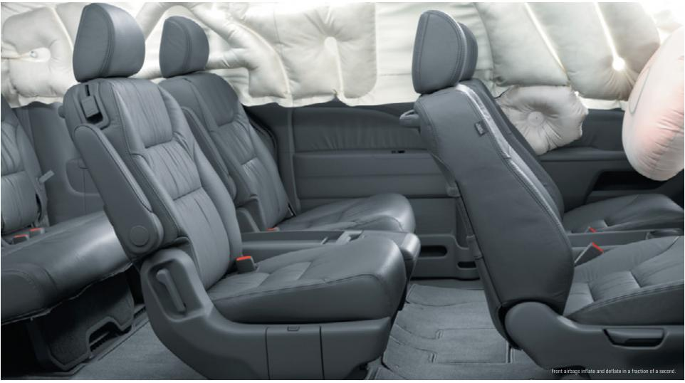
Front airbags,\* front side airbags and 3-row side curtain airbags with a rollover sensor are standard. The dual-stage, dual-threshold front airbags deploy at one of two rates and thresholds depending on the severity of impact and seat-belt use. Sensors prevent the deployment of the passenger's side airbag if a child or small adult is in the airbag's deployment path.
