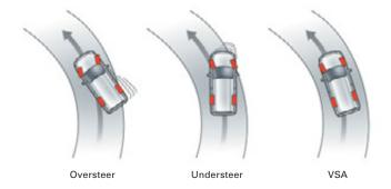
All 2005 Odysseys now feature Honda's sophisticated Vehicle Stability Assist (VSA) system. Working with ABS and electronic throttle control, VSA **enhances stability** by detecting oversteer or understeer, and braking individual wheels and/or reducing throttle to help restore the driver's intended path of travel.
