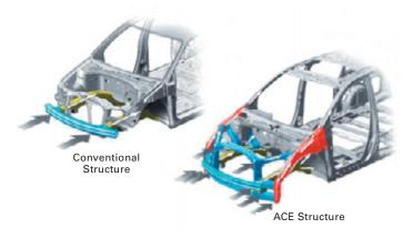
Honda's Advanced Compatibility Engineering (ACE) body structure incorporates a front-end frame structure that absorbs and disperses crash energy over a larger area. ACE increases Odyssey passenger protection, and makes it **more crash-compatible** with vehicles of differing ride heights.
