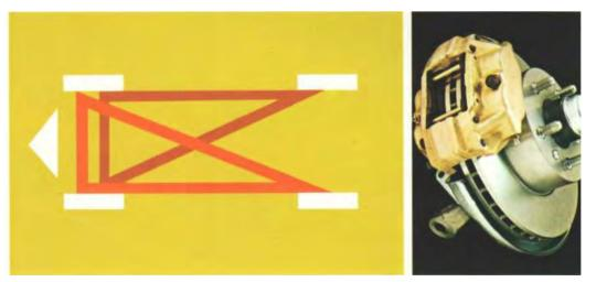
The Volvo 164E has 4-wheel self adjusting power disc brakes and two separate braking systems. Each operates on the two front wheels and one rear wheel. Since each front brake furnishes 30% Of the car's total braking power while each rear wheel supplies 20%, you always have 80% of the car's braking power working for you even if one system fails. Brake system
