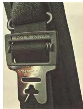
The Volvo self-adjusting safety belt is comfortable to wear. It unwinds from an inertia reel when you put it on. You'll find one for every corner passenger.
