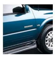
Help protect your vehicle from unsightly side nicks and scratches with running boards.†† Custom-designed, they feature a durable aluminum substructure that is both corrosion- and rust-resistant.
