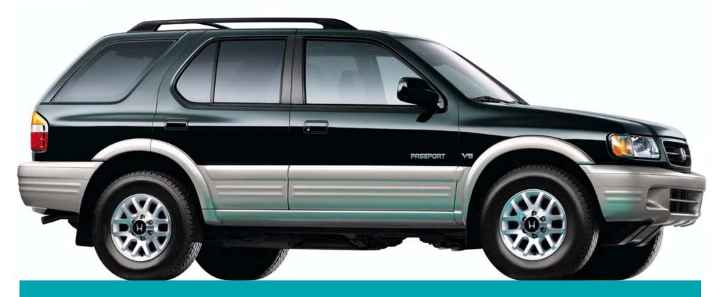
Versatile, capable and tough, the Passport has been engineered from the ground up for an active lifestyle. Its 205-hp, 3.2 liter, 24-valve engine produces 214 lb.-ft. of torque and also runs so clean that the Passport qualifies as a Low-Emission Vehicle (LEV).
