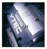
A 200-hp, 2.2 liter, 16-valve, DOHC VTEC 4-cylinder engine gives the Prelude its high-revving power. Dual overhead camshafts allow the valves to be more optimally placed, resulting in increased power. Prelude's **4 valves per cylinder** assure the cylinder deep breaths of air and fuel. The more you pack in, the more power you get out. They also quickly and more thoroughly purge the cylinder of spent exhaust gasses.
