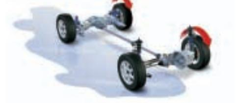
If one or both wheels on one side of the car spin, more power goes instantly to the wheels on the opposite side with the best traction.
