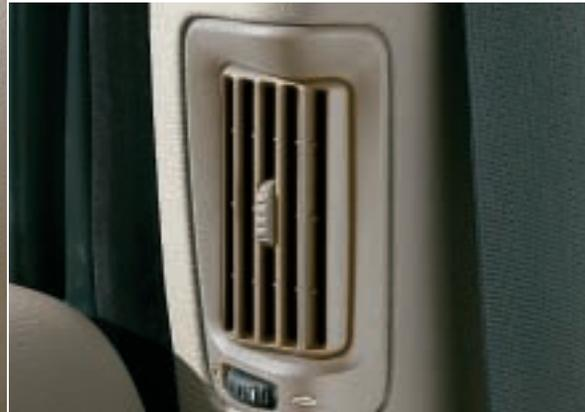
Adjustable air vents for the rear-seat passengers further enhance comfort and help keep the side windows from fogging.
