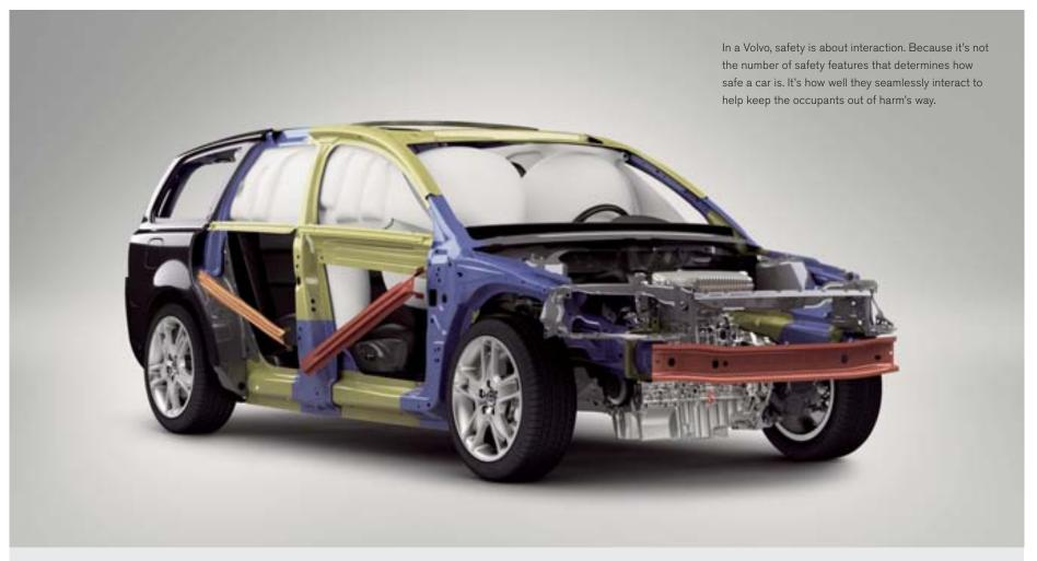
In a rear impact the rear deformation zones will help absorb crash energy. The fuel tank is designed to remain well protected in front of the rear axle. The head restraints help protect the neck and spine, and Volvo's unique Whiplash Protection System (WHIPS) cradles the front seat occupants in a controlled manner to help prevent whiplash injuries.
