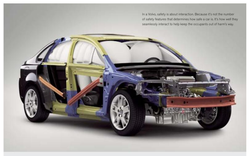
In a rear impact the rear deformation zones will help absorb crash energy. The fuel tank is designed to remain well protected in front of the rear axle. The head restraints help protect the neck and spine, and Volvo's unique Whiplash Protection System (WHIPS) cradles the front seat occupants in a controlled manner to help prevent whiplash injuries.
