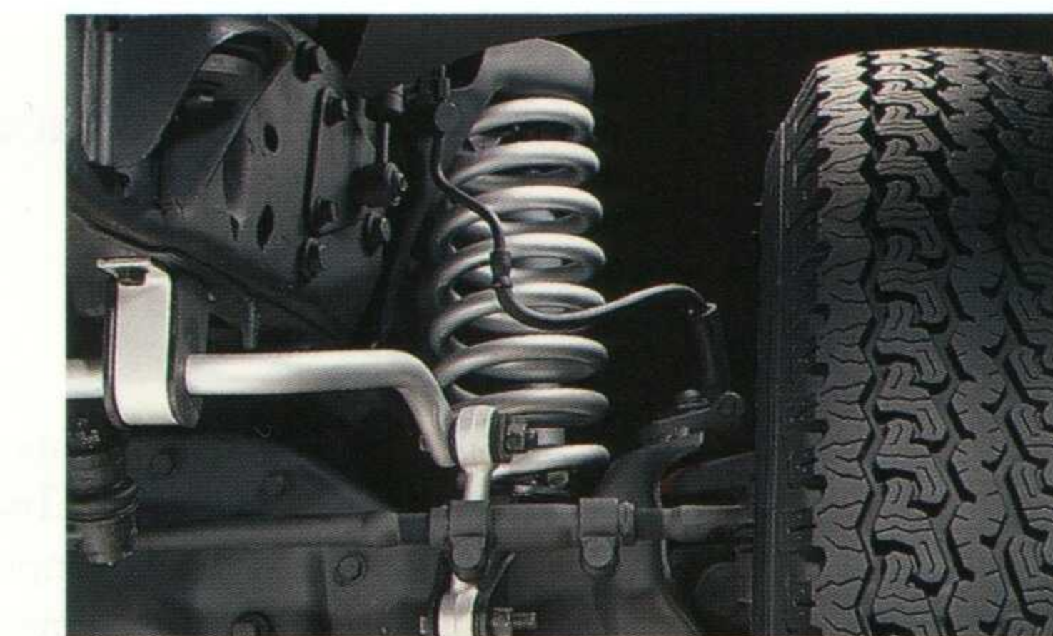
◀ Independent front suspension is very surefooted in rough terrain.
