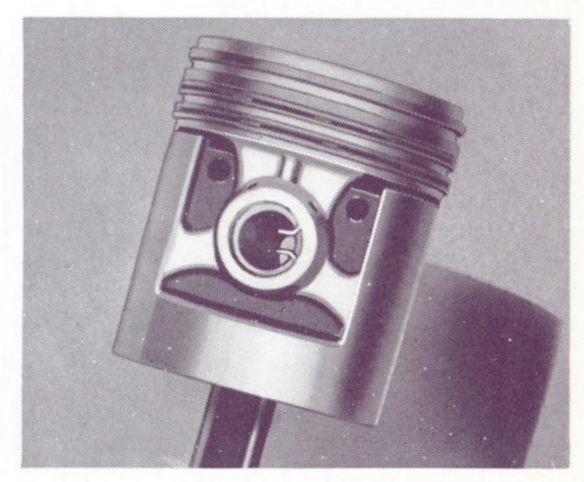
Aluminum alloy pistons with four rings instead of the usual three are used.
