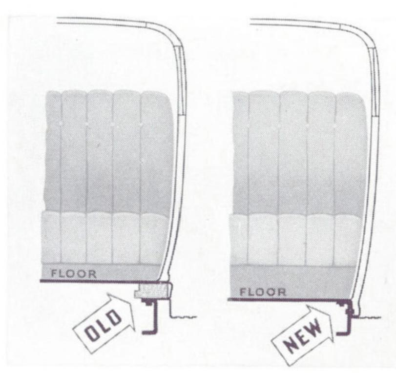
The Dodge all-steel body fits down over frame instead of being mounted on top. More head-room without increasing over-all height.
