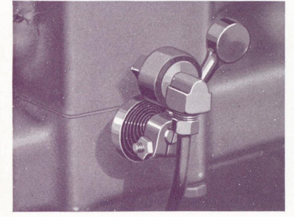
A manifold heat control heats the fuel for smoother operation when the engine is cold.
