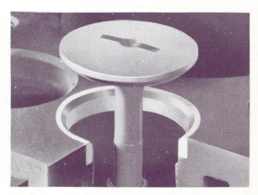
Tool steel exhaust valve seat inserts save fuel and defer valve grinding many miles.
