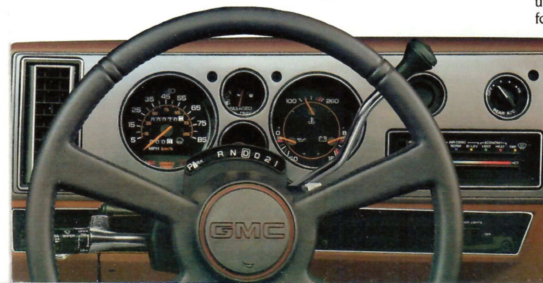
Instrument cluster features full-gage package and electric speedometer
