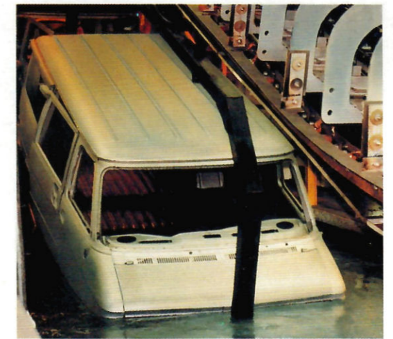
The entire body is immersed in electrically-charged primer
