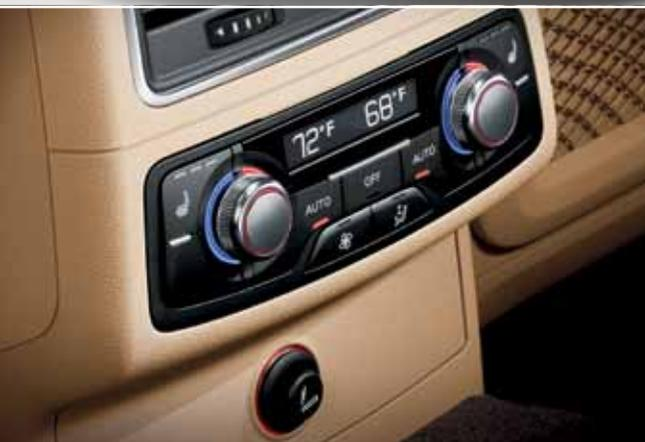
**Four-zone, automatic climate control** | Occupants in the driver and front passenger seats, as well as the occupants of the outer rear seating areas, can select and control their desired level of heating or cooling via the center console. A light sensor on the dashboard adjusts the system based on the sun's intensity.
