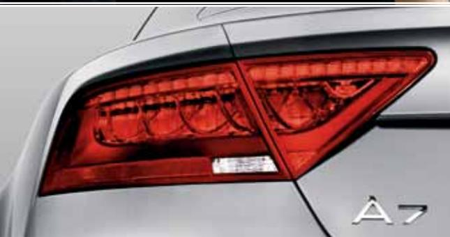
**LED taillights** | LED lights are superior to conventional bulbs thanks to faster activation speeds and bright light emissions. In addition, they can last an entire vehicle lifetime and consume up to 50 percent less energy while adding a signature look to your Audi.
