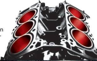
VCM can activate and deactivate the engine's cylinders as needed, so you enjoy brisk acceleration while also maximizing fuel efficiency. And the transitions between modes are seamless to the driver.
