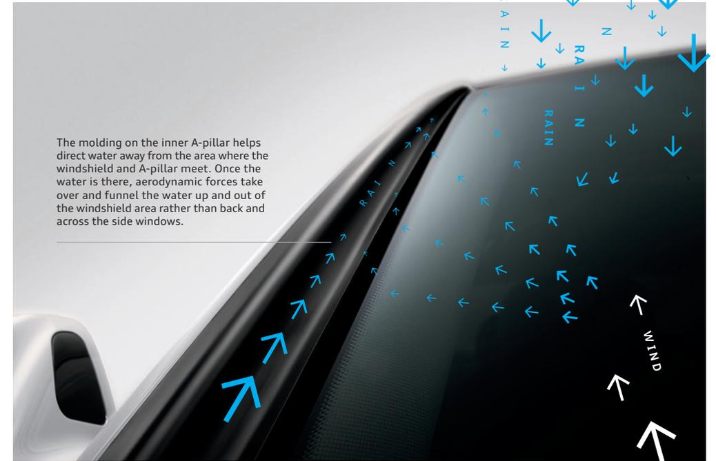
The molding on the inner A-pillar helps direct water away from the area where the windshield and A-pillar meet. Once the water is there, aerodynamic forces take over and funnel the water up and out of the windshield area rather than back and across the side windows.
