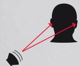
Unlike with high-frequency sounds, the brain cannot detect where low bass frequencies are coming from, making it seem as if the sound is hitting both ears at the same time. Because of this, Bang & Olufsen® sound engineers only had to design one custom-fitted subwoofer to reproduce the kind of deep, cabin-filling bass that brings music to life.
