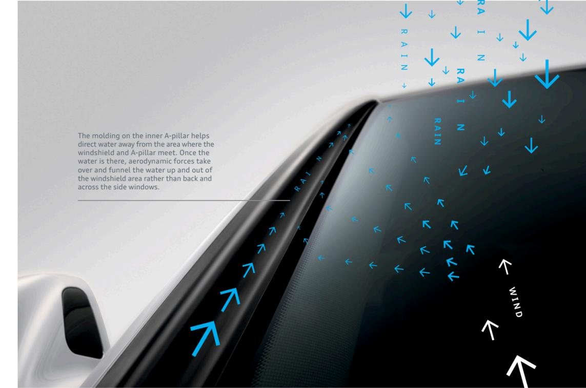
The molding on the inner A-pillar helps direct water away from the area where the windshield and A-pillar meet. Once the water is there, aerodynamic forces take over and funnel the water up and out of the windshield area rather than back and across the side windows.
