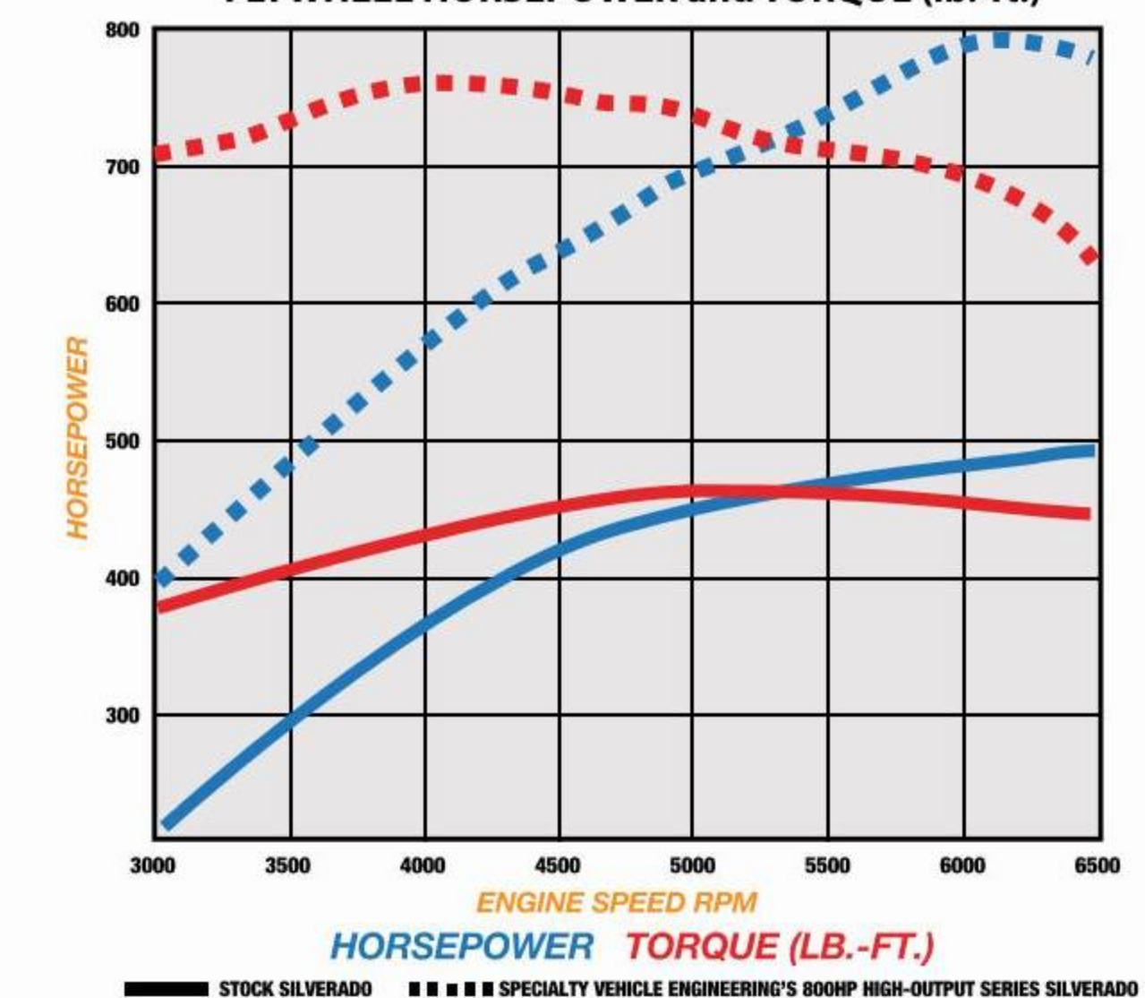
2018 800HP 6.8L HIGH/OUTPUT SERIES SILVERADO FLYWHEEL HORSEPOWER and TORQUE (lb.-ft.)
