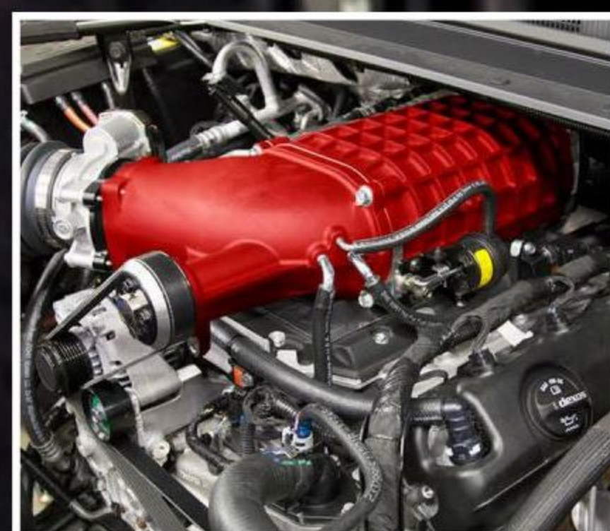
Specialty Vehicle Engineering's High/Output Series supercharged engine with 800 horsepower and 750 lb.-ft of torque makes this 2018 Yukon one of the fastest SUVs on the road. Shown with optional supercharger paint (black is standard).
