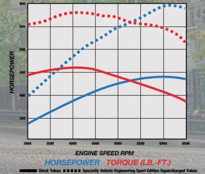
2018 575HP 6.2L SPORT EDITION SUPERCHARGED YUKON FLYWHEEL HORSEPOWER and TORQUE (lb.-ft.)
