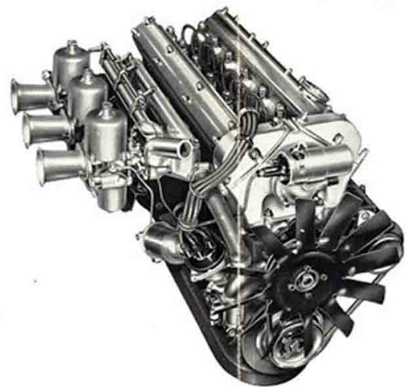
The engine fitted to the "S" type model incorporates "straight port" cylinder head which, combined with three HD8 SU carburetors and 9:1 compression ratio, gives a power output of 250 b.h.p. at 5,500 r.p.m.
