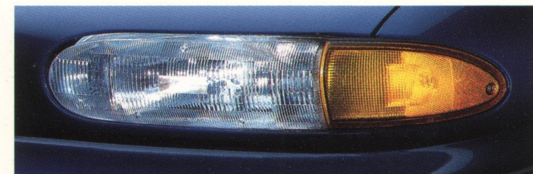
← A BRIGHT IDEA: FLUSH MOUNTED HALOGEN HEADLAMPS.
