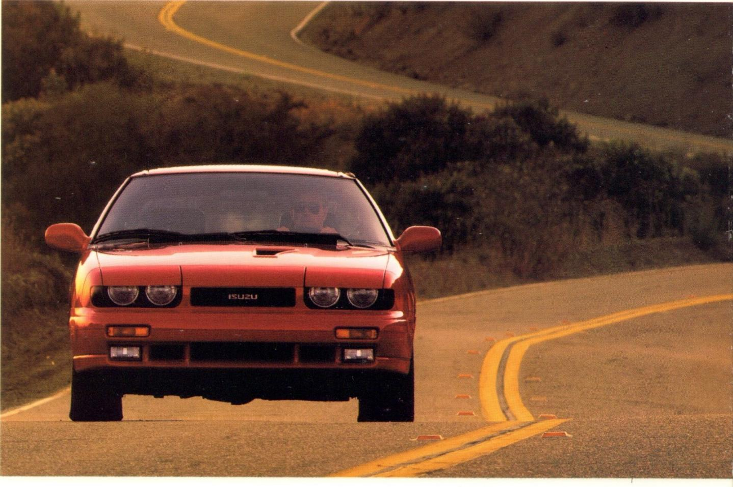
The highly sophisticated full-time all-wheel drive system found on the high-performance Impulse RS divides the engine's impressive power 43/57 to the front and rear wheels for optimum performance. Viscous couplings dramatically improve acceleration and handling in all conditions by diverting power to the wheels with the best traction.
