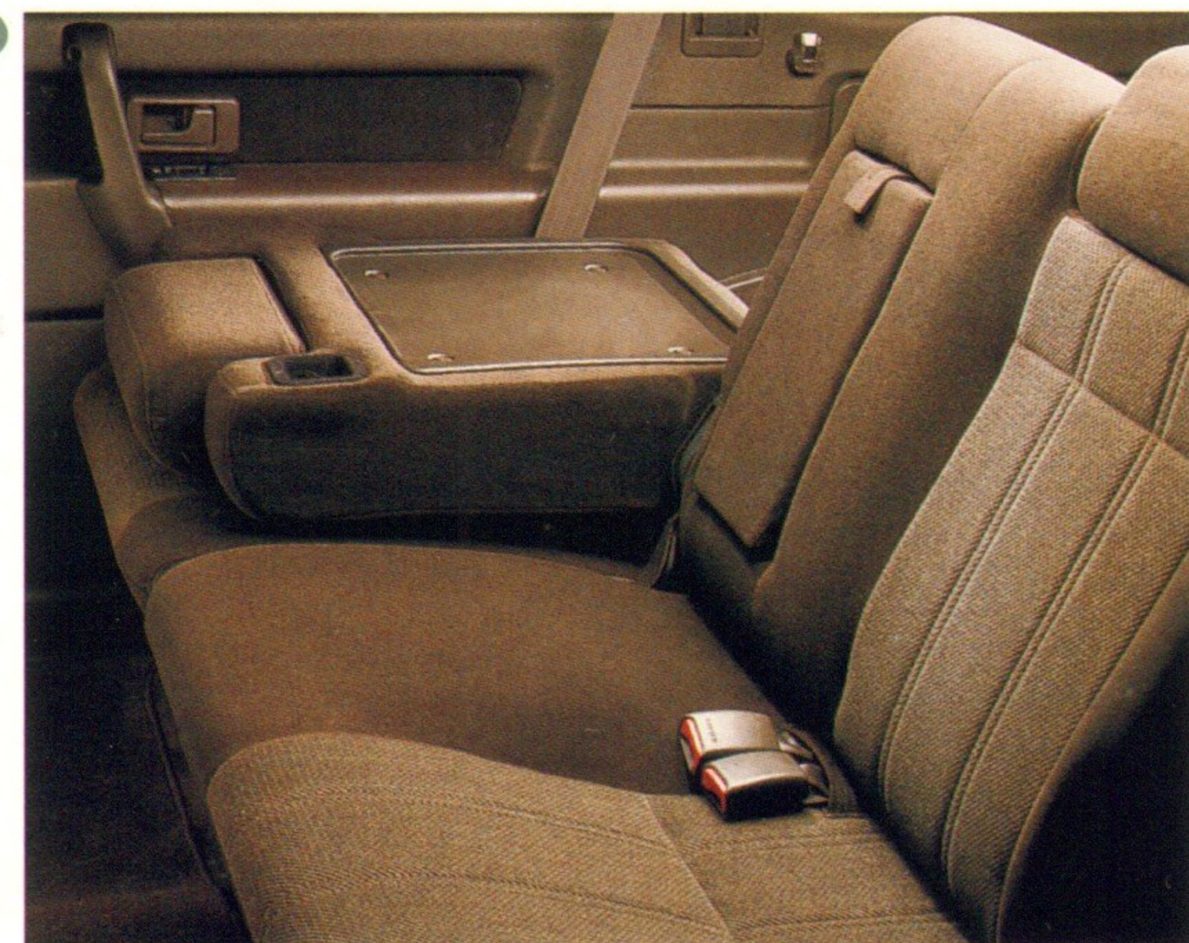
1 The 60/40 split rear seat features an armrest, adjustable head restraints, and seatbacks that recline up to 40 degrees. (Standard on Trooper LS, optional on Trooper S.)
