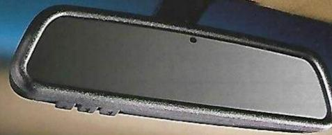
**HOMELINK** Besides automatically dimming at night when headlights hit it, Axiom's electrochromic rearview mirror has an integrated HomeLink® Universal Transceiver which can be programmed to open garage doors, security gates, even turn on house lights.
