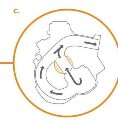
at lower RPMs. C. The valve rotates to an open position, creating a shorter intake that provides maximum torque and performance at higher speeds.
