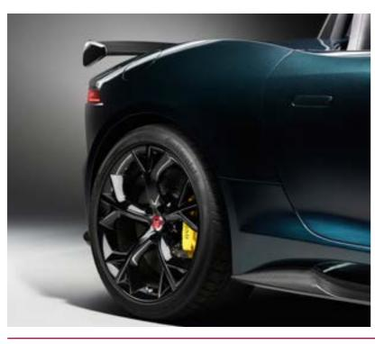
The rear deck, bonnet vents, side vent louvres and mirror caps are also all made of carbon-fibre. The windscreen length is reduced by 114mm, reducing overall height by 30.5mm, with new side windows to match the profile.
