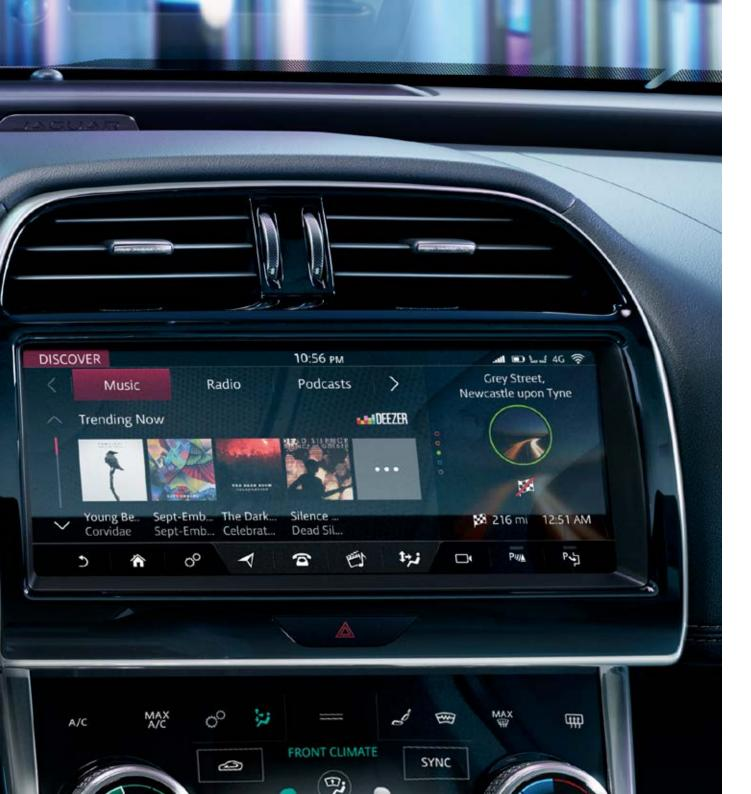
Touch Pro Duo<sup>1</sup> is our innovative twin-screen system, part of Jaguar InControl<sup>®</sup> technologies, providing a 10" upper Touchscreen and 5.5" lower Touchscreen. The benefit of having a lower screen is to allow dual-tasking, for example, navigation mapping on the upper screen and climate controls and access to other features – such as entertainment – on the lower screen<sup>\*</sup>.
