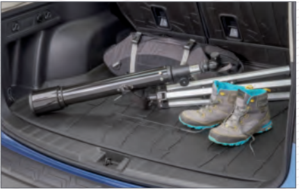
Cargo Tray. Helps protect the trunk area from stains and dirt while providing a surface that helps reduce the shifting of cargo while driving.
