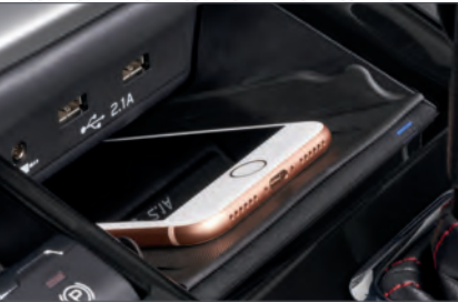
Wireless Charger. Conveniently charge your phone without the hassle of tangled wires. The Wireless Charger is a Qi Certified Device with Intelligent Charging Profiles, cell phone battery protection, temperature control technology and short circuit safe guards. Compatible with all Qi enabled devices and Samsung Fast Charge enabled devices. Anti-Slip rubber insert safely holds your mobile device.
