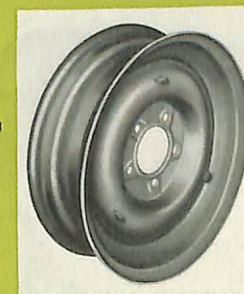
Balanced wheels with drop center type rims.
