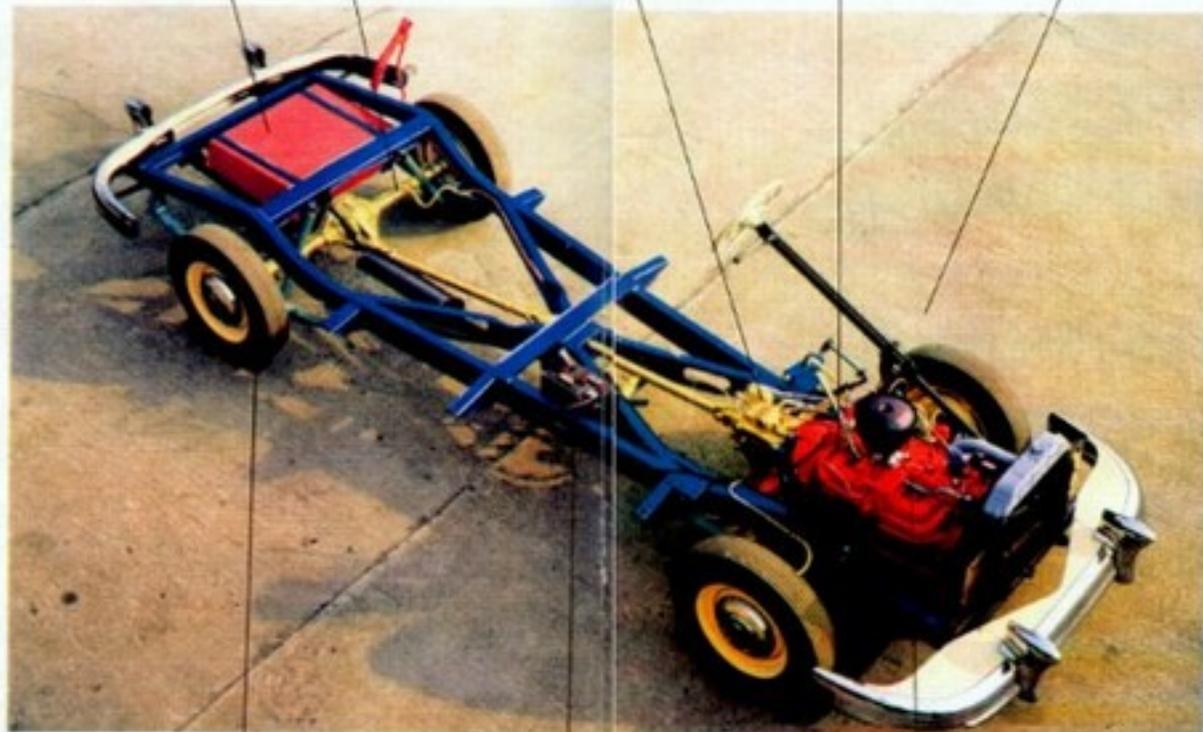
**BRAKES.** Wagner hydraulic, self-centering, self-adjusting shoes adjust automatically to compensate for lining wear
