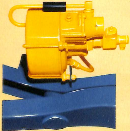
POWER BRAKES— Extra large; bonded lining; master cylinder under hood.
