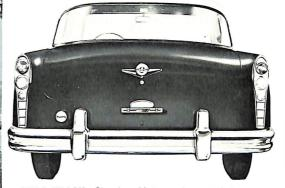
WIDE TRACK—Checker Motors pioneered the use of the wide track and has perfected its performance. Cornering is as nimble as with a sports car. Bigger 15" wheels mean larger brakes, more brake lining area, and longer life to tires and brakes.
