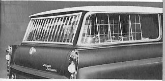
te Aerobus luggage compartment is partitioned off from the assenger area for additional passenger comfort and load carryge convenience. Horizontal and vertical strips of stainless steel event damage to windows and to the luggage.
