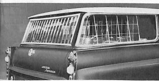
re Aerobus luggage compartment is partitioned off from the assenger area for additional passenger comfort and load carryg convenience. Horizontal and vertical strips of stainless steel event damage to windows and to the luggage.
