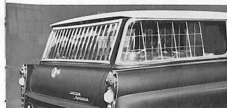
The Aerobus luggage compartment is partitioned off from the passenger area for additional passenger comfort and load carrying convenience. Horizontal and vertical strips of stainless steel prevent damage to windows and to the luggage.
