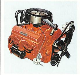
Now, choose from 3 greatly improved—most proven—engines. A standard 140 HP, 230 cu. in. economy overhead valve six; an optional 195 HP, 283 cu. in. regular gas V-8; a new 327 cu. in. 250 HP high performance V-8 ideally suited to trailer towing, also optional.
