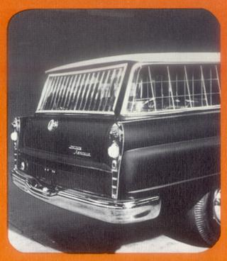
The huge Aerobus luggage compartment with room enough for a dozen or more pieces of large luggage plus many other parcels, can be partitioned off from the passenger area with plexiglass (optional). Horizontal and vertical strips of chrome plated copper (optional) prevent damage to windows and to the luggage.
