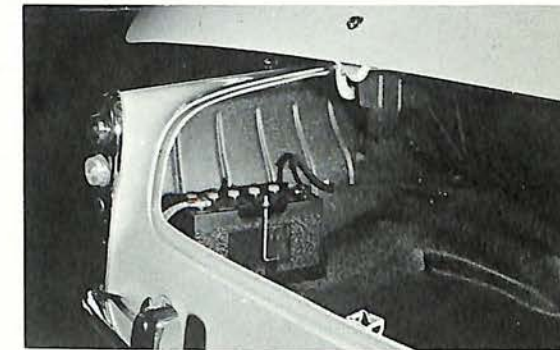
Rear Mounted Battery Many operators now prefer the rear mounted battery option since engine heat frequently will affect length of battery life. Counter-balanced trunk lid shown in illustration is standard equipment.
