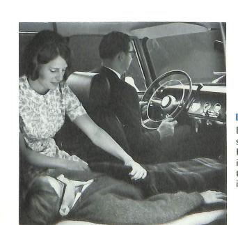
**Driver Comfort** Bucket-type seat is standard for driver. Each passenger is visible. Photo shows interior with stretcher in position.
