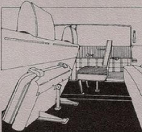
5. Square, forward-facing auxiliary seats are available in A-12E as an option. Allows for up to six passengers in rear compartment.
