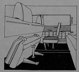
5. Square, forward-facing auxiliary seats are available in A -12E as an option. Allows for up to six passengers in rear compartment.
