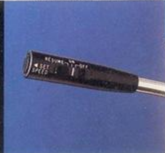
21. "Auto-Cruise". Maintain constant speed without touching the accelerator pedal for effortless highway driving, better fuel economy. Holds any pre-selected speed above 30 mph ± 2 mph depending on vehicle and road condition variables.
