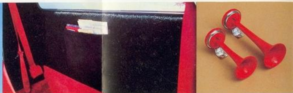
18. Carpet Kit. "Poly-Velour" carpet material in this kit adds insulation and sound absorption to the Pickup cab's interior. Center piece has sewn-in map pocket. Available in colors to match or complement cab interior. Installs with adhesive.
