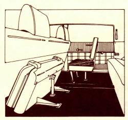
Square, forward-facing auxiliary seats are available in A-12E as an option. Allows for up to six passengers in rear compartment.
