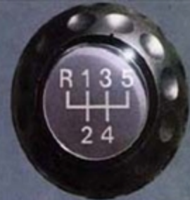
5-speed manual with 4th/5th overdrive ratio.
