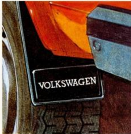
SPLASH GUARDS: Made of lightweight, molded ethylene vinyl acetate copolymer and available with silver logos.
