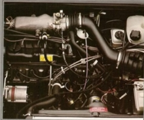
1.8 liter fuel-injected overhead cam engine—performance tuned.
