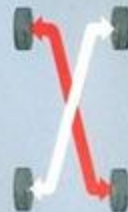
Scirocco's dual diagonal braking circuits help assure safe stops.
