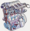
GM's 2.0 liter fuel injection engine features the standard technology of a fuel-injection "flexible design." Each cylinder has its own intake valve, maximizing the engine's power response throughout the range.
