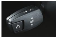
■ Dynamic Cruise Control lets you store and keep to a chosen speed above 20 mph, automatically applying the brakes downhill. It is activated via the left-hand steering column switch, and deactivated by applying the brakes or via the switch.<sup>3</sup>
