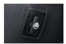
**Heated steering wheel** is a feature that, like heated seats, becomes a "must-have" once it's experienced. The heating switch is conveniently located on right-hand side of the steering column.
