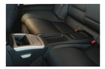
■ Rear Console provides rear-seat occupants with ample storage, both open and covered, and climate controls for rear-cabin airflow rate and temperature. The center fold-down armrest contains two retractable cupholders.
