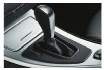
☐ 6-speed STEPTRONIC automatic transmission provides a choice of three modes: "Drive" with Adaptive Transmission Control; a more dynamic "Sport" mode; and STEPTRONIC automatic, for the hands-on control of a manual without a clutch.¹
