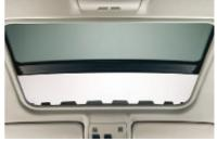
■ Two-way power glass moonroof with remote, expanded one-touch operation, slides forward or tilts up to let in as much fresh air and sky as you like, while a wind deflector helps keep the wind out. Includes a sliding interior sunshade.
