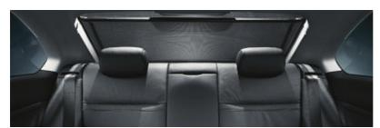
□ Power sun shade for the rear window can be conveniently raised and lowered. This feature helps eliminate glare, maintains occupant privacy, and helps keep the cabin temperature pleasant by reflecting intense sunlight.
