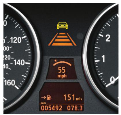
□ Active Cruise Control allows the driver to set a desired speed that is automatically maintained in free-flowing traffic. However, as the 3 Series Coupe approaches a slower-moving vehicle ahead, a radar sensor in the front bumper alerts the system. Active Cruise Control will then act to match the speed of the slower vehicle, and remain a set distance behind, pre-selected by the driver. As soon as the lane ahead is clear, Active Cruise Control automatically returns the car to the set speed.¹
