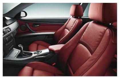
Eight-way adjustable front sport seats with two-way manual headrests and thigh support make the driving experience more enjoyable. Side bolsters can be power-adjusted to fit your back comfortably while helping to hold you firmly in place during cornering. (328i models require optional power seats or Premium Package)
