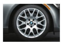
Cross Spoke (Style 197) light alloy wheels and run-flat<sup>2</sup> performance tires.<sup>3</sup> In front: 18 x 8.0 wheels and 225/40 tires; in back: 18 x 8.5 wheels and 255/35 tires. (328i Sport Package; opt. on 328i xDrive, requires optional Sport Package)
