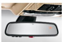
The automatic-dimming inside rear-view mirror darkens in response to the bright headlights of vehicles behind you. The easy-to-read digital compass, integrated into the mirror, is a convenient way to constantly keep your bearings while driving. A three-button Universal garage-door opener can be programmed to open garage doors and activate various remote convenience functions.
