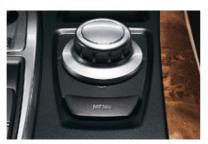
■ iDrive Controller, conveniently located on the center console, allows access to a variety of functions that are displayed on the Control display screen. The turn/press button enables front-seat occupants to access the menu system and fine-tune settings for climate control, the audio system, Navigation system<sup>4</sup> and communication through BMW Assist.™1
