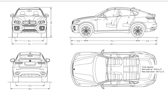
All dimensions of the technical drawings in inches. Height indicated with roof antenna and unloaded.
