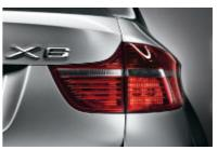
■ Adaptive Brake Lights increase vehicle visibility and signal the intensity of your braking action, thereby warning following drivers to brake quickly.
