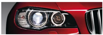
■ Xenon Adaptive Headlights optimize road illumination when the X6 enters a turn or corner, helping to enhance visibility when driving at night. Sensors continuously monitor the angle of the steering wheel to determine the direction in which the X6 is heading. The outer headlights swivel accordingly, up to 15 degrees left or right.
