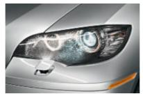
Retractable, high-intensity headlight washers help keep lights clean of ice, mud, road salt and other coatings, for maximum road lighting and enhanced driving visibility.
