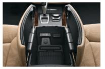
iPod and USB adaptor lets you scroll through and select music by using the vehicle's radio controls, the multi-function steering wheel buttons or the iDrive Controller. Music titles are displayed on the radio or screen. Auxiliary input port lets you connect an external audio source, such as an iPod or MP3 player.
