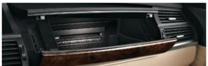
**DVD** changer, located in the glovebox, accommodates six discs, as well as single-feed. The easily accessible six-disc changer supports multi-channel sources, and plays compressed audio formats (MP3, WMA, etc.). When equipped with the Navigation system, the DVD changer can also play video on the iDrive screen when the vehicle is stationary.
