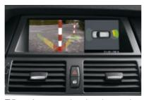
□ Rear-view camera is activated automatically by shifting into reverse gear, or manually by pressing the parking-assist button. The color display shows a real camera image that may include "static" and "track" lines to help you when backing up or parallel parking. (optional; included in the X6 xDrive35i Technology Package)
