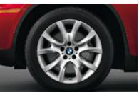
■ 19 x 9.0 V-Spoke (Style 257) light alloy wheels and 255/50 run-flat all-season tires are standard on the X6 xDrive50i. (Run-flat tires do not come equipped with a spare tire and wheel.)
