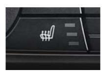
Heated front seats are a welcome feature for driver and front passenger in cooler weather. With the touch of a button, the seat surface and backrest are heated and quickly radiate comfortable warmth in your choice of three settings.
