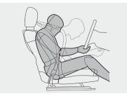
BMW restraint system for the driver and front passenger combines three-point safety belts, automatic safety-belt pretensioners, seat bolsters that help prevent occupants from sliding forward, and head restraints. This system helps provide optimum restraint in a collision.
