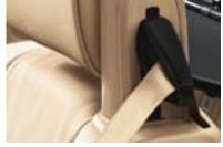
■ Seat-integrated front safety belts help keep occupants firmly and comfortably in place. The seat-integrated design also helps ease entry and exit for rear-seat passengers.
