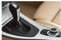
☐ 6-speed STEPTRONIC automatic transmission provides a choice of three modes: ☐ Drive☐ with Adaptive Transmission Control; a more dynamic ☐ Sport☐ mode; and STEPTRONIC automatic, for the hands-on control of a manual without a clutch.
