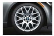
Cross Spoke (Style 197) light alloy wheels with run-flat<sup>1</sup> performance tires.<sup>2</sup> In front: 18 x 8.0 wheels with 225/40 tires; in back: 18 x 8.5 wheels with 255/35 tires. (328i Sport Package)
