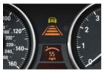
☐ Active Cruise Control system uses radar measurements to automatically maintain a preset speed and distance between your vehicle and the one ahead in highway driving.1
