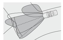
Xenon Adaptive Headlights illuminate the road ahead and to the side with brilliant clarity; Xenon headlights also have a dynamic autoleveling feature. BMW Adaptive Headlights illuminate the road around corners by directing the headlights into and through the bend, as soon as the vehicle begins cornering.
