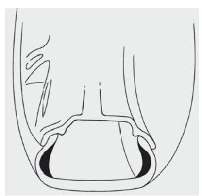
**Run-flat tires** allow speeds of up to 50 mph and travel from 30 to 150 miles after a loss of air pressure, depending on the passenger load and weight of articles being transported. In situations that would normally result in a flat tire, reinforced sidewalls help prevent the tires from collapsing or loosening from the rim. In the event of a decline in tire pressure, the driver is warned by the **Tire Pressure Monitor**.
