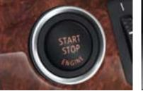
■ Engine Start/Stop button<sup>3</sup> and remote key control the engine. First, insert the remote key into the starter switch slot. After the electronic identification system confirms that it is the correct remote key, you can start (or later, turn off) the engine by pressing the Start/Stop button.
