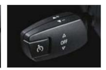
■ Dynamic Cruise Control lets you store and keep to a chosen speed above 20 mph, automatically applying the brakes on a downhill. It is activated via the left-hand steering column switch and deactivated by applying the brakes or via the switch.²
