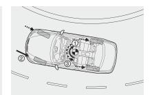
Cornering Brake Control increases vehicle stability by proportioning the braking force while turning. When you brake in a turn, the pressure comes off the rear wheels, which causes the vehicle to swerve inward (oversteer) (1) Cornering Brake Control counteracts this action by asymmetrically adjusting brake pressure (2), creating stabilizing countertorque (3), independently of the ABS system.
