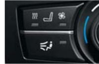
Front seat ventilation gently blows warm air or cool air through the microperforations in the leather to help keep driver and front passenger comfortably dry in hot weather, and warm in colder weather.
