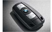
☐ Comfort Access system offers an even greater degree of convenience: keyless access to your vehicle. Simply carrying the remote key in a pocket allows you to unlock the doors by touching the door handle. You can also turn the engine on or off by pressing the Start/Stop button without inserting the remote key. (Foot must be on brake in order to start.)
