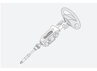
Telescoping steering column system. In a collision, a section absorbs a portion of the impact force and collapses, helping
