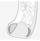
Run-flat tires allow speeds of up to 50 mph and travel from 30 to 150 miles after a loss of air pressure, depending on the passenger load and weight of articles being transported.<sup>1</sup> to protect the driver. In situations that would normally result in a flat tire, reinforced sidewalls help prevent the tires from collapsing or loosening from the rim. In the event of a decline in tire pressure, the driver is warned by the Tire Pressure Monitor.
