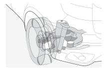
Tire Pressure Monitor is an electronic control system designed to warn the driver if there is a sudden and irregular loss of tire pressure. Should the target pressure of a tire fall below 25%, a warning light alerts the driver.
