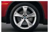
☐ Star Spoke (Style 259) 20 x 10.0 front, 20 x 11.0 rear light alloy wheels with 275/40 front and 315/35 rear run-flat¹ performance tires² are available as an option when ordering the X6 xDrive50i Sport Package and Sport Activity Package. (Not available on X6 xDrive35i.)
