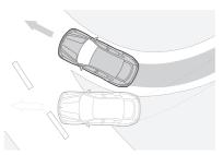
Dynamic Stability Control provides remarkable tenacity on slippery road surfaces. If the system senses over- or understeer, it modulates engine power and can apply brakes individually to help keep the vehicle under control and going in the intended direction.
