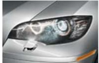
Retractable, high-intensity headlight washers help keep lights clean of ice, mud, road salt and other coatings, for maximum road lighting and enhanced driving visibility.
