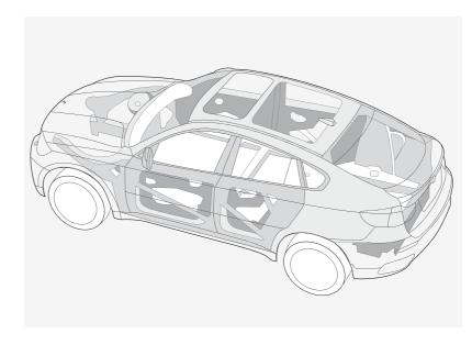
Extremely rigid body creates a protective safety cell that directs severe impact forces around the passenger compartment. Thanks to BMWIs intelligent lightweight design and the use of high-strength steels, the interior passenger compartment is surrounded by a stronger shell than was previously possible to construct.
