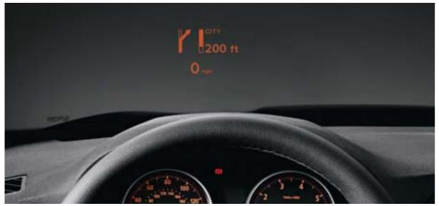
☐ **Head-up Display** projects important travel information, such as current speed, on the windshield directly in the driverIs line of vision. Directional arrows from the Navigation system and Check Control data can also be displayed.
