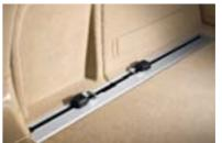
Storage package adds practical extras: additional lighting and two lashing rails with four sliding lashing eyes.
