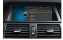
■ Glare-free Control display screen, linked with the iDrive and Navigation system, renders clear images and text. The surface of this new-generation display is equipped with transreflective technology, ensuring legibility by automatically making adjustments to the brightness or background lighting in brightor poor-light conditions.
