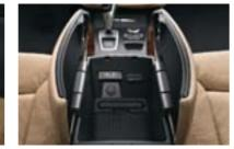
iPod and USB adapter lets you scroll through and select music by using the vehicle's radio controls, the multi-function steering wheel buttons or the iDrive Controller. Music titles are displayed on the radio or screen. Auxiliary input port lets you connect an external audio source, such as an iPod or MP3 player.
