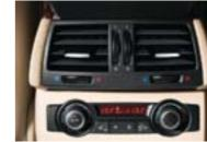
Four-zone climate control lets occupants, both front and rear, select individual temperature and fan settings.
