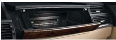
**DVD changer,** located in the glovebox, accommodates six discs, as well as single-feed. The easily accessible six-disc changer supports multi-channel sources, and plays compressed audio formats (MP3, WMA, etc.). When equipped with the Navigation system, the DVD changer can also play video on the iDrive screen when the vehicle is stationary.
