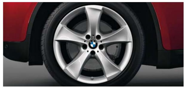
Star Spoke (Style 259) 20 x 10.0 front, 20 x 11.0 rear light alloy wheels with 275/40 front and 315/35 rear run-flat1 performance tires<sup>2</sup> are available as an option when ordering the X6 xDrive50i Sport Package and Sport Activity Package. (Not available on X6 xDrive35i.)
