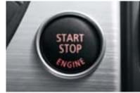
■ Engine Start/Stop button and remote key control the engine. First, insert the remote key into the starter switch slot.
