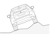
Rollover sensor, linked with the Dynamic Stability Control system, quickly detects when the X6 is at risk of rolling over and assists the driver in maintaining control of the vehicle. If a rollover is imminent, the airbags and the safety-belt pretensioners are immediately triggered to provide additional occupant protection.
