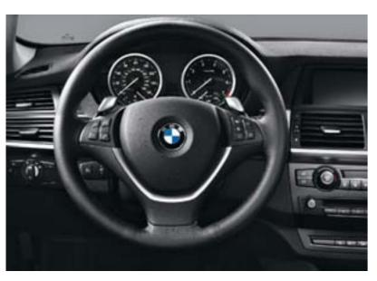
■ Three-spoke leather-wrapped multifunction sport steering wheel, featuring power tilt/telescoping adjustments, lets you keep both hands on the steering wheel while adjusting both the audio and a BMWapproved, Bluetooth® enabled mobile phone.
