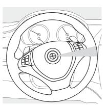
Greater agility at low and medium speeds: With Active Steering, a small turn of the steering wheel translates into a big turn of the front wheels.
