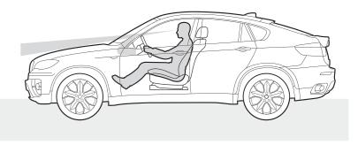
The Head-up Display shows relevant information, such as the carls speed, directly into the driver's field of vision. The height-adjustable display helps keep you focused on what's happening on the road.
