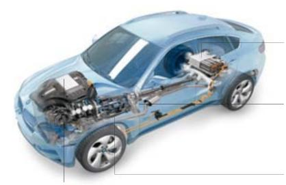
**Electric air conditioning compressor:** The electric drive of the air conditioning system runs independently of the combustion engine. You can create a comfortable climate and maintain it while driving on electric power alone  $\mathbb I$  or even when the engine is switched off. This leaves more hybrid energy available for other uses, and full use of all hybrid functions  $\mathbb I$  even during sporty driving and in extreme weather.
