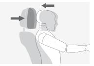
Active Head Restraints in the front seats reduce the risk of whiplash or neck/head/ spine injury. When sensors detect a rearend collision, the headrests rapidly and automatically pivot forward, supporting the driver s and front-seat occupant heads.
