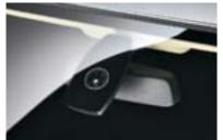
■ Rain sensor uses infrared light to measure the amount of rain. When the wipers are in the <code>□</code> intermittent <code>□</code> mode, the rain sensor automatically adjusts the windshield-wiping interval as needed. Automatic headlight control (not shown), included with rain sensor, activates headlights by means of a sensor that responds to darkness.
